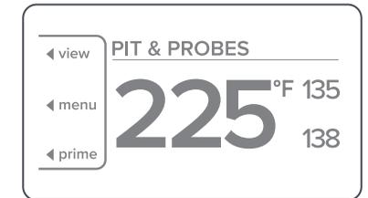
As shown in Section 1.C, the “Pit & Probes” view is the default display option. There are five total display options; they can be chosen by pressing the view selection button on the control panel.
