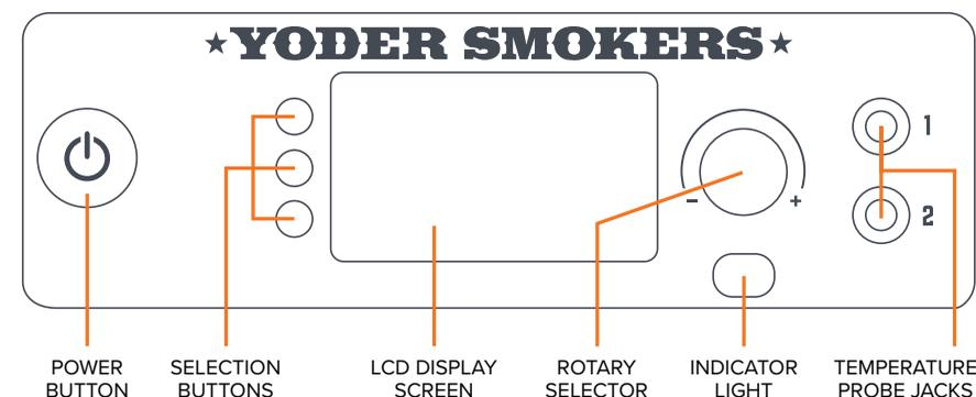
**POWER BUTTON** – Powers the grill on and off. Once the grill is turned on, and a fire has started, pressing the power button to turn the unit off will initiate shut down mode. This mode allows the fans to continue running to ensure a safe, full burn of any pellets left in the firepot. The unit will turn off once the grill reaches 125°F or runs for 18 minutes, whichever occurs first.
