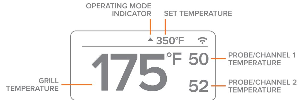
**GRILL TEMPERATURE** – Displays the current temperature of the grill at the center of the main cooking surface. Upon startup, the temperature displayed will be the set temperature until the internal temperature of the unit reaches 125°F. At that point, the controller will display the temperature of the main cooking surface.
