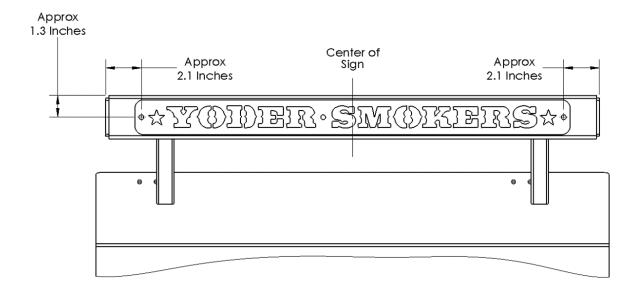
Center the sign on the counterweight then mark the hole location through the sign preferably with a center punch. Use a #7 bit to drill the holes then thread them using a ¼-20 NC tap. Secure the sign with the provided stainless button head cap screws.
