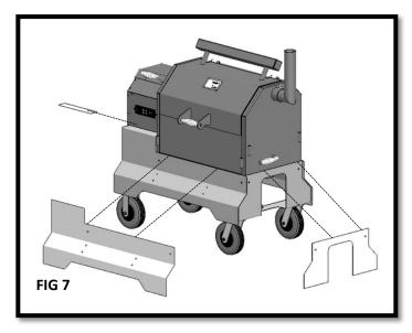
5. Install the back panel and hopper end panel by aligning the top edge of the magnet panel to the top edge of the comp cart. Starting from the top, smooth out the wrap to fit the contours of the panel and ensure all bolt holes line up. Center the hopper trim panel to the top side of the cart next to the hopper. If you are having issues with the back panel not fitting to the contour of the cart, try warming up the surface with a hair dryer as previously mentioned. (FIG 8)
