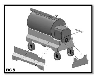
the wrap line up with the holes in the cart, and that all pieces are properly located. Insert the power cord extension through the opening of the comp cart and plug the cord into the hopper. (FIG 9) Then secure the power socket using the Phillips screwdriver and 5/16" wrench. (FIG 10) \*NOTE\* if you removed the 3 wires from the power socket in step 3, refer to (FIG 11) for wire installation to power socket.
