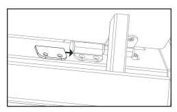
**Step 10** – Install and hand-tighten (2) of the 3/4" long Flat Head Phillips supplied in kit through chamber with #10 Flange Nuts removed in Step 7, as shown.
