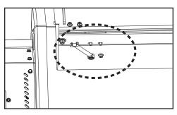
**Step 8** – Remove the (2) Flat Head screws from hinge closest to the hopper.
