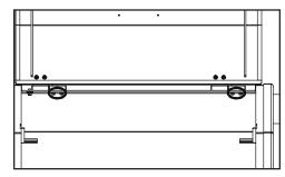
Step 7 – Using 3/8" Wrench, loosen and remove flange nuts from hinge closest to the hopper, as shown. Set these aside for reassembly.
