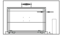
**Step 4** – Find the 1/2" wide x 29-1/2" long Seal Strips, and adhere (1) along the top and (1) along the bottom of lid, as shown.
