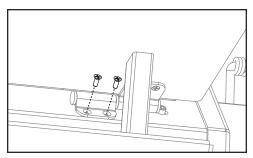
**Step 9 – WITH THE AID OF ANOTHER PERSON**, slightly lift the lid and slide the shim under the hinge and align holes, as shown.
