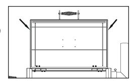
**Step 6** – Inside the cooking Chamber, locate #10 Flange nuts below hinges.
