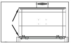
**Step 5** – Find the 1/2" wide x 21-1/2" long Seal Strips. Adhere (1) to the left side and (1) to the right side of the lid, as shown.
