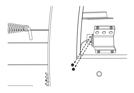
Feed the thermocouple wire through the hold on the chamber wall and into the hopper. Using the screws and nuts from the previous step, install the short thermocouple into the same the holes in the chamber from the previous thermocouple.
