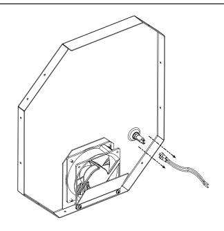
Disconnect the Wi-Fi extension wire from the controller using a small adjustable wrench.
