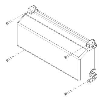
Carefully remove the box from the controller by sliding the harness through the slot in the box.
