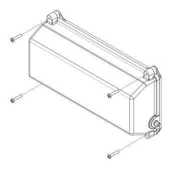
Install the ACS controller into the hopper and secure it in place using the two screws removed from the faceplate.
