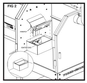
Using a 1/8" allen wrench, loosen the set screws that hold the igniter in place. NOTE: DO NOT REMOVE THE METAL HOUSING AROUND THE IGNITER.
