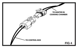
5. Gently pull on the igniter cable wire assembly to remove the igniter from the igniter tube.
