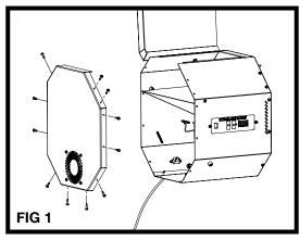
2. Disconnect the two wires (one green, one white) from the fans. (Make a note of which fan terminal gets green, and which gets white).
