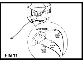
13. Reconnect wiring spade terminals to fan.
