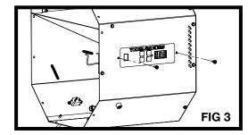
4. Pull out control box and spread it open to gain access to the wiring on the back side of the green circuit board.
