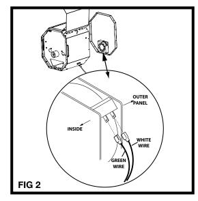
3. Using a 5/16" socket, remove two 1024x12 controller bolts that secure the control box to the hopper.
