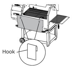
Locate the two hooks on the inside face of the front blanket. These are secured to the exposed front edge of the cooking chamber. Two notches in the blanket fit around the two front shelf mounting cylinders.
