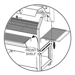
Next, remove the front shelf (can be left off until blanket installation is completed)
