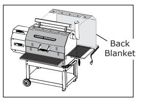
Blanket is slotted to fit around arms of counterweight. Front edge of blanket slides under top blanket and twist tabs fit into mating slots in top blanket. Rotate tabs 90° to lock in place.
