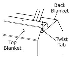
With top and back blankets secured to one another, final step is to fasten lower belts of back blanket to lower belts of front blanket. Adjust for a snug fit.
