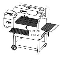
First, raise the lid to the cooking chamber, exposing the front edge of the chamber.
