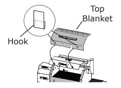
Two hooks on underside of blanket fasten to lower edge of raised lid. Two notches in the blanket slide over handle brackets; Yoder Smoker logo faces up; eyelets for attaching back blanket are facing up.
