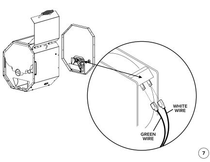
Ensure all wires are free of both fans and the auger drive motor. Lastly, attach the end panel to the hopper using the eleven self-drilling screws.
