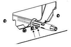
5. Attachignitercable at electrical connector. Tuck the wire backins ide the hopper away from firepot.
