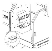
2. Use the 5/16" socket and extension to remove the igniter housing from the chamber wall.
