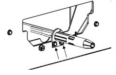
3. Pull the wires out of the opening to the hopper to expose the electrical connector. Pull apart the electrical connector for the igniter
