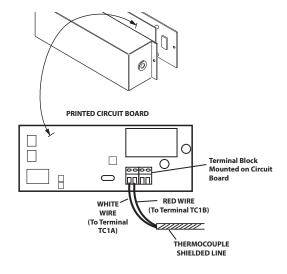
7. Route the thermocouple wires through the grommet of the control box and reattach to the black terminal block on the green circuit board (white wire to terminal TC1A; Red wire to terminal TC1B).
