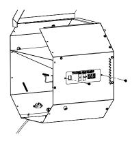
10. Reconnect wiring spade terminal to the fan.
