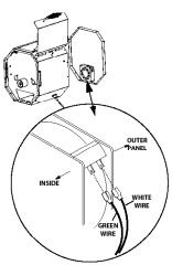
11. Reassemble hopper end panel using eleven 10x34 self-tapping screws.
