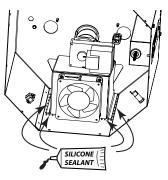
**6**. Reconnect wiring spade terminals to the fan.
