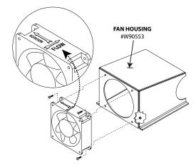
**5**. With fan assembly positioned in place, use the silicone sealant supplied with the installation kit to secure the fan housing to the floor of the hopper (in illustration below, arrows indicate the areas around the housing base requiring silicone sealant).
