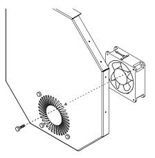
**4**. View showing fan assembly positioned under th∉ auger motor assembly:
