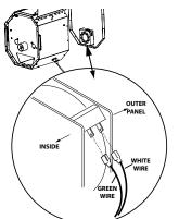
3. Remove two front panel screws
