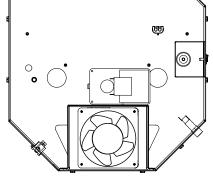
**2**. Attach fan to new fan housing (p/n W90553) using four screws (#8-32x1/2" phillips head machine screws) and nuts (#8-32). NOTE: Fan must be installed with Air Flow Arrow on top of fan pointing toward the fan housing (see inset, below).
