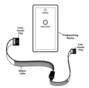
6. First, insert the 6 pin female plug of the ribbon cable onto the 6 pin terminal block of the control box circuit board. Correct orientation is with the red wire of the cable "up", as shown (wire closest to the blue transformer).
