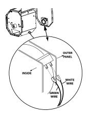
**3**. Remove two front panel screws.
