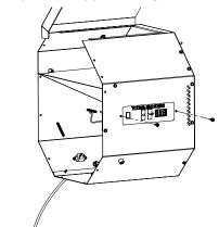
**11**. Reconnect wiring spade terminals to fan.
