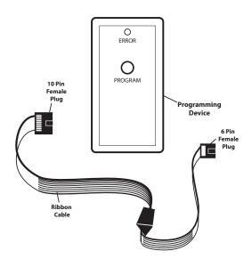
6. First, insert the 6 pin female plug of the ribbon cable onto the 6 pin terminal block of the control box circuit board. Correct orientation is with the red wire of the cable "up", as shown (wire closest to blue transformer)
