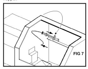
Route the thermocouple wires through the grommet of the control box and re-attach to the black terminal block on the green circuit board (white wire to terminal TC1A; red wire to terminal TC1B).
