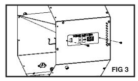
Pull out control box and spread it open to gain access to the wiring on the back side of the green circuit board.
