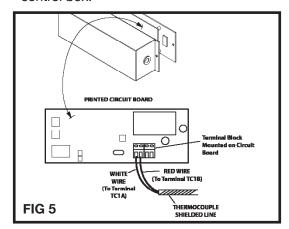
Remove thermocouple from mounting bracket by unscrewing #6-32x1.5" screws and nuts. Save screws for installation of new thermocouple. Gently pull thermocouple wires out of hopper through hole. See FIG 6.
