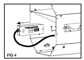
Disconnect two thermocouple wires on the green circuit board using a small blade screwdriver (FIG 5). Pull these wires out of the control box.
