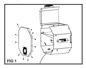
2. Disconnect two wires (one green, one white) from the fan. (Make a note of which fan terminal gets green, and which gets white).
