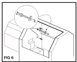
7. Secure new thermocouple in mounting bracket with the two #6-32x1.5" screws and nuts. Then feed thermocouple wire back through hole into hopper.
