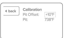
8. The offset temperature will be highlighted to indicate that it is entered. You may now press the back button multiple times to return to the main screen.
