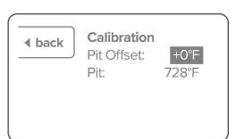
7. You will no longer see the temperature highlighted. Rotate the selector knob clockwise to increase the offset and counterclockwise to decrease the offset. Press the selector knob once you have the desired temperature offset to confirm the changes.
