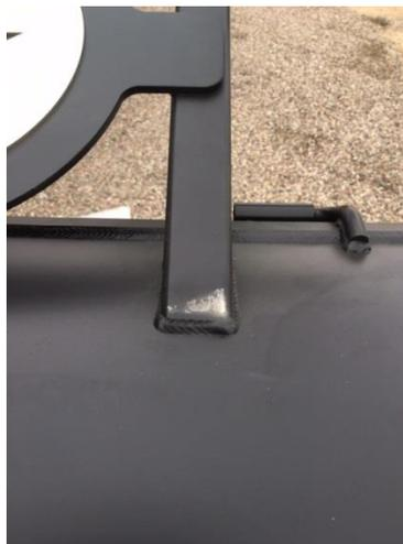
After further investigation of the plastic wrap and foam, a small slit was found where the damage occurred. The following pictures show that a small slit through the plastic and the foam were directly over the damaged area. This was caused from something coming in contact with the cooker during shipping.
